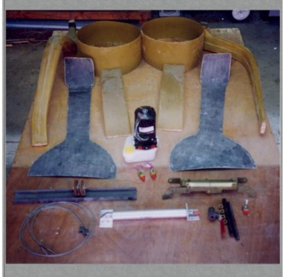
The retrofit kits as per picture are available and will include the main gear legs, gear doors, gear wells, special over center device, hydraulic pump & cylinder, and special miscellaneous hardware. The kits are made to fit Long EZs or Cozys. Approximate cost is \$3,000. Complete installation of kit is also available. For more information or the \$25 video please email Steve Drybread or call 1-
