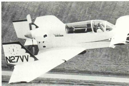
Burt Rutan's VariViggen. Plans for this aircraft have been approved by NASAD and have been rated "Amateur, Average." This means that, in NASAD's opinion, the VariViggen can be built as a first time project by persons having only the common hobby shop power tools and hand tools. The prototype now has over 400 hours of flying time logged and copies are being built in 10 different nations. Look for some very exciting developments from the Rutans in the months ahead.
